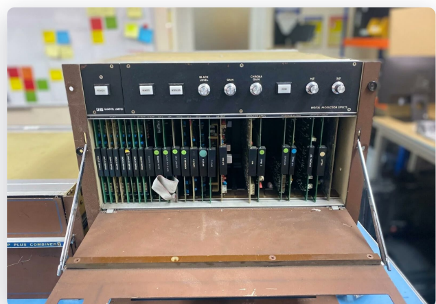
The chassis open: the row of “FRAME STORE” cards — the picture memories that changed everything.
